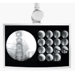
A 24" landscape splitscreen monitor or dual 19" monitors can be attached to existing wall or ceiling support arms to increase flexibility and save OR space. (Ceiling support arm is not provided by Ziehm Imaging)
