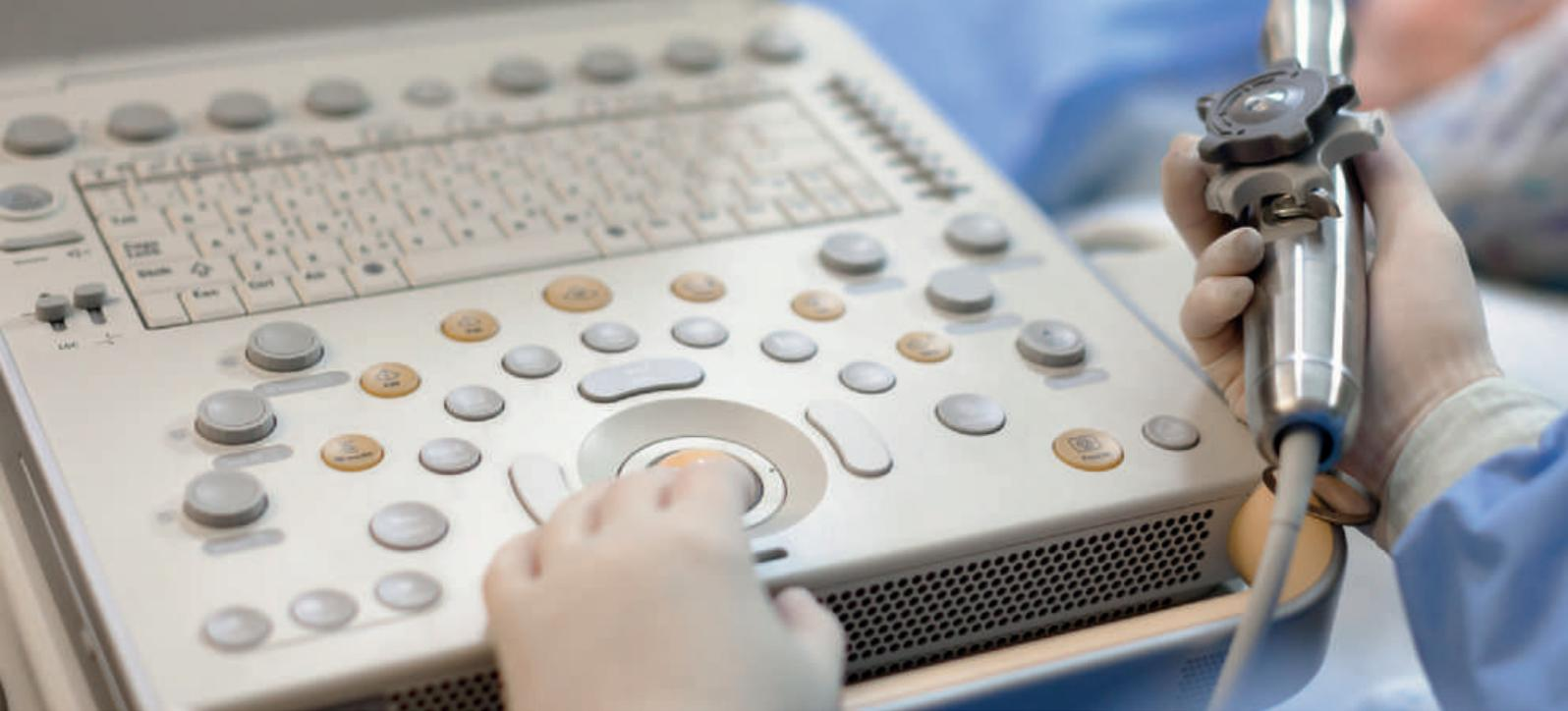
One-button controls are logically placed on the CX50 control panel for quick selection and optimization during every exam. An example: iSCAN automatically samples data for quick optimization of 2D and Doppler performance.
